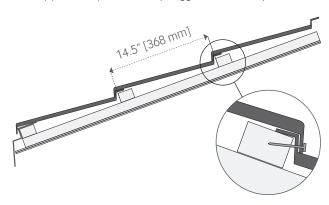
Panels are placed on nominal 2x2 wood battens spaced 14.5" [368mm].
