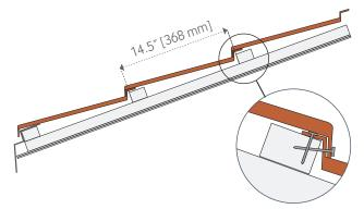
Panels are placed on nominal 2x2 wood battens spaced 14.5" [368mm].
