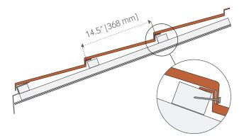
Panels are placed on nominal 2x2 wood battens spaced 14.5" [368mm].
