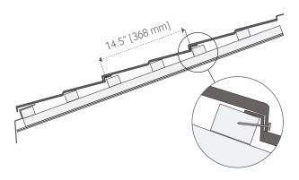
Panels are placed on nominal 2x2 wood battens spaced 14.5" [368mm].
