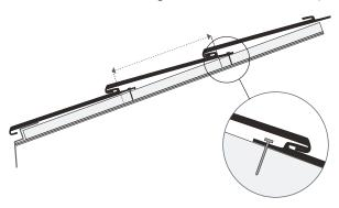
The panels are placed onto deck spaced 14.5" or 368 mm.
