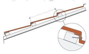
The panels are placed onto battens spaced 14.5" or 368 mm.
