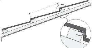
The panels are placed onto battens spaced 368 mm or 14.5".
