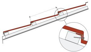
The panels are placed onto battens spaced 368 mm or 14.5".
