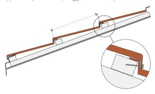
The panels are placed onto battens spaced 368 mm or 14.5".
