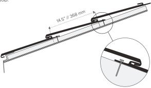
The panels are placed onto deck spaced 14.5" or 368 mm.
